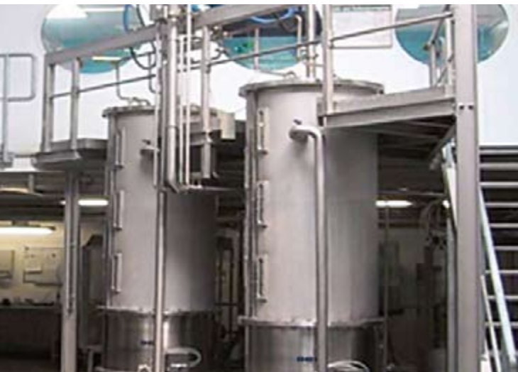
Figure: patented EBA chromatography columns used for purification of HANNILASE® XP
